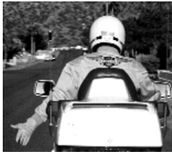
Arm extended down. Palm forward. Swing forward from hip in arc.
